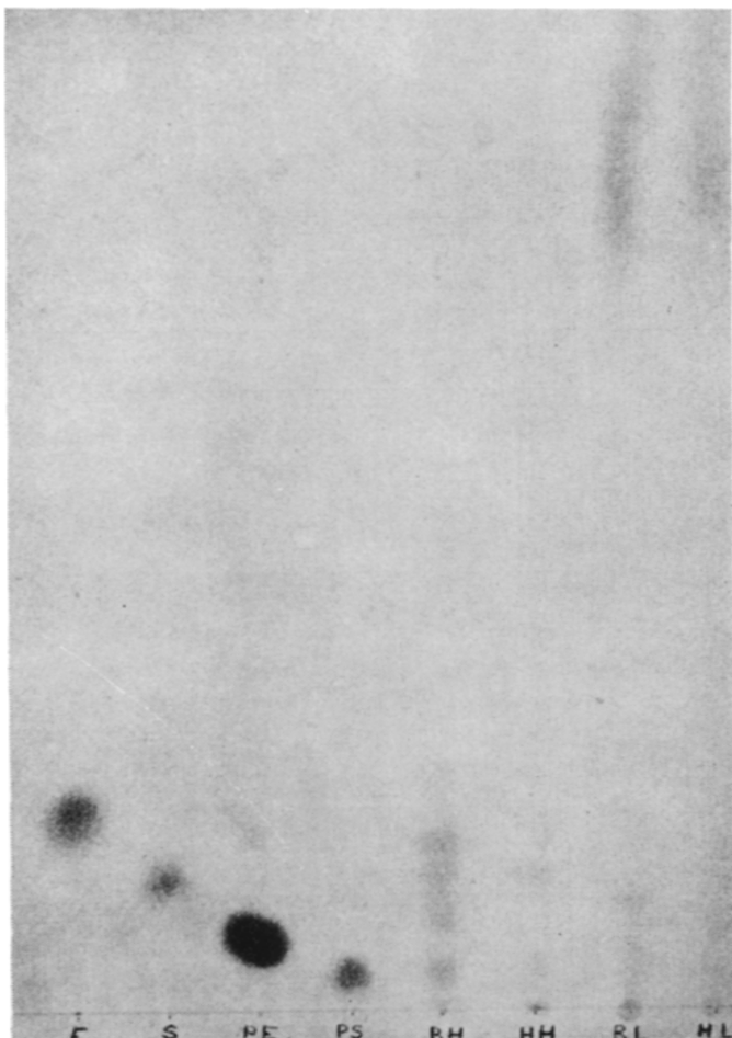
Fig. 1. Amino-acid paper chromatography of lipid extracts and their hydrolysates stained with ninhydrin. (E) = Ethanolamine; (S) = serine; (PE) = phosphoethanolamine; (PS) = phosphoserine; (RH) = hydrolysate of rabbit plasma lipids; (HH) = hydrolysate of human plasma lipids; (RL) = rabbit plasma lipids; (HL) = human plasma lipids. Extracts of 1 ml plasma applied.
